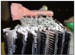
Image 9: Part of the work the battery testing facility does is to subject batteries to simulated accelerated life cycle testing with post mortem failure analysis. As example, the cell failure due to material shedding and short circuiting of a lead acid starter battery after testing is shown in the picture
