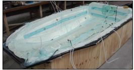
Image 7: Vacuum infusion setup used to introduce infusion as viable technology for boat building within the CIC programme
