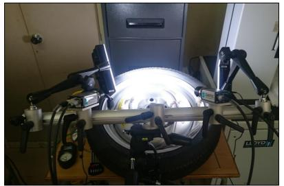
Image 5: Digital Image Correlation equipment used on a spare wheel strain gauged in order to validate the FE model under both an inflation test as well as a dynamic fatigue test.
