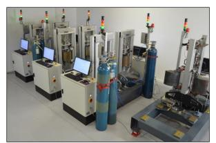
Image 14: Small Punch Creep Testing Facility based on NMMU South campus
