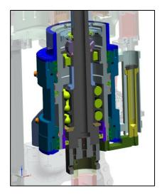
Image 1: Design of the in-house commissioned WC4 Boss Welding Machine mounted on a modelled specimen
