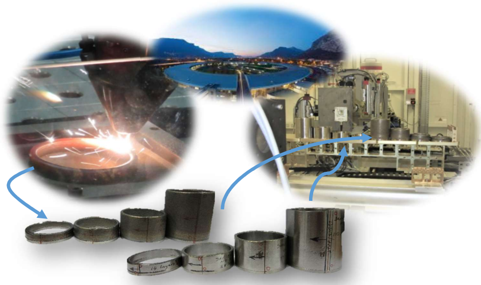
LMD manufactured Ti6Al4V parts evaluated on Beam line ID15 at the ESRF facility in Grenoble France.
