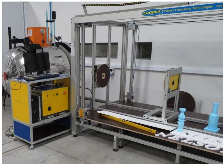
Hot-Wire Cutter and Autoclave
